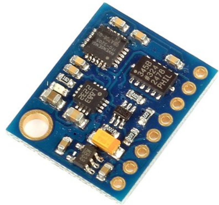
GY-85 chipset (9 axis orientation sensor)
